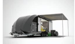
↑ Awning can be fitted on either or both sides
